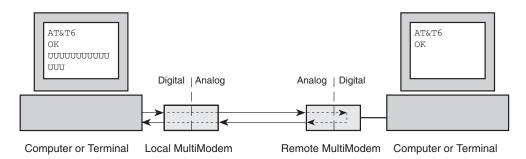
Figure C-2. Remote digital loopback test.
